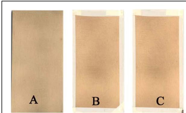
*Figure 4. BronzeShield™: Accelerated weathering on polished bronze.*
