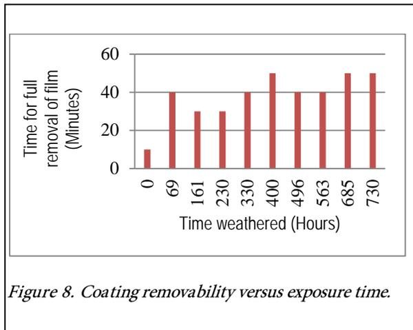
Figure 8. Coating removability versus exposure time.
