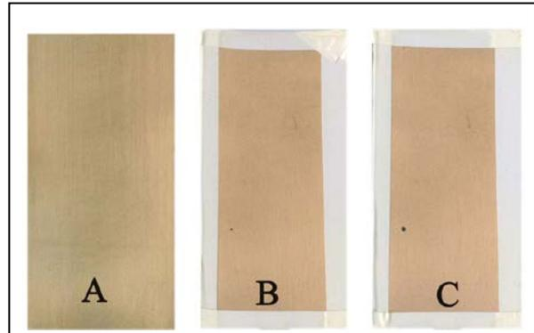
*Figure 6. Incralac: Accelerated weathering on polished bronze.*
