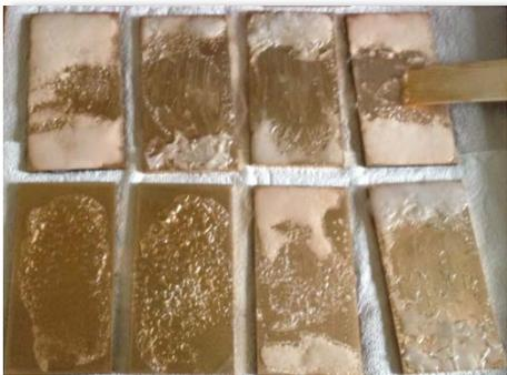
*Figure 3. BronzeShield™ samples being tested for removability.*
